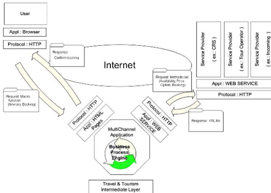
**Fig. 4.** The general architecture of the ROBINTUR system
